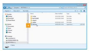
If the PC programme does not start automatically, start Windows<sup>®</sup> Explorer, open the KEYTOOLS drive and start the programme by double-clicking on "start.exe".
