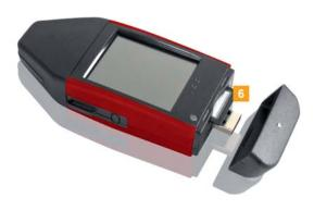
6 If you require a backup copy, insert an SDHC™ card into the card slot.
