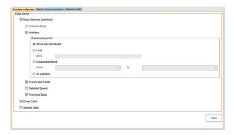
In the **Configuration** module on the **Download configuration** tab, specify the data you want to download from the digital tachograph.
