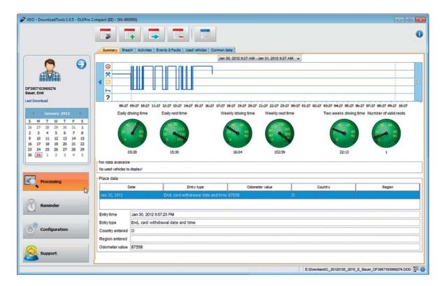
The **Viewer** module offers you a number of tabs with which you can analyse the downloaded mass memory and driver card data – either in detail or in the form of a summary.
