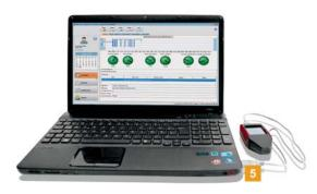
5 If possible, leave the DLKPro plugged into the computer when you finish working with it – this will charge the integrated rechargeable battery e. g. for the next card download.
