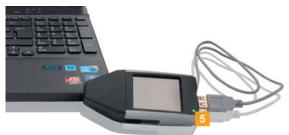
5 Check that the data transfer to and from the DLKPro has finished: The LED light remains green.
